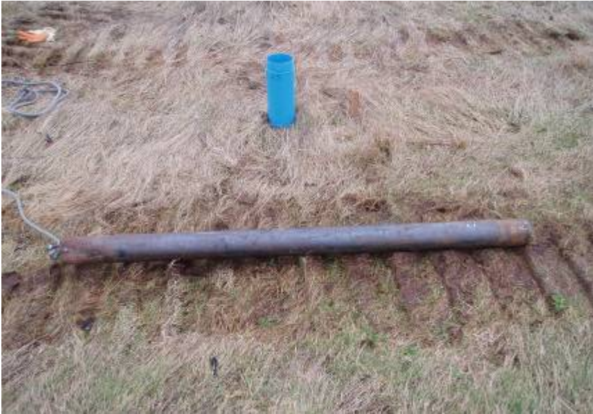
Down-hole high-resolution gamma probe ready for deployment
