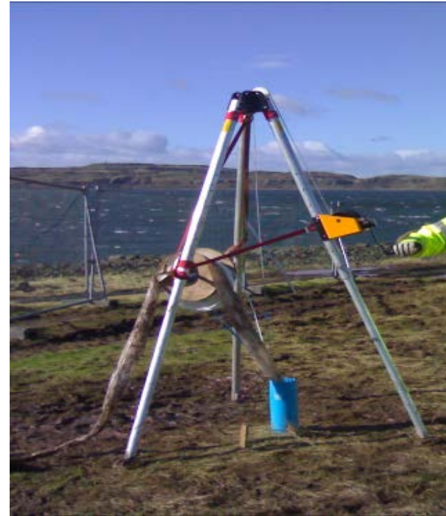
Probe deployed in temporary borehole
