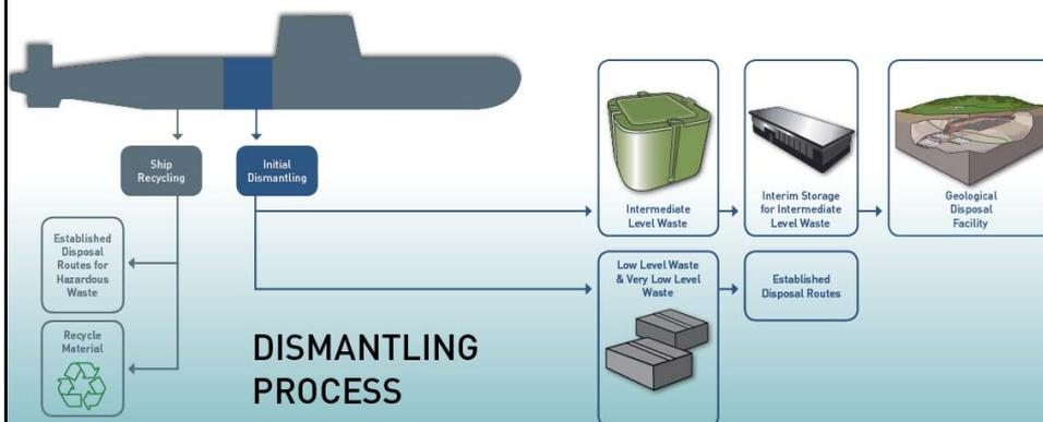
Figure 6: Dismantling Process
