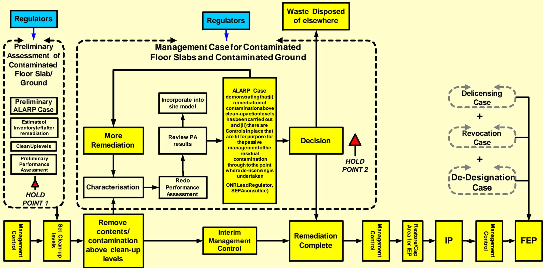
**Generic Route Map for deciding the End State of Contaminated floor slabs and Contaminated ground through to the Final End Point**
