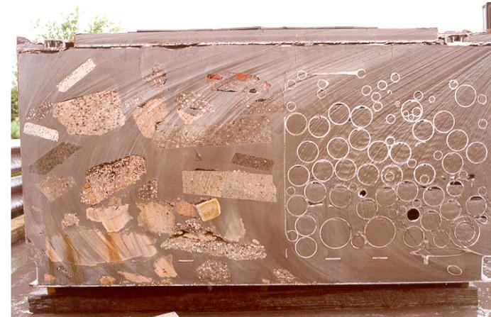
Decommissioning waste infilled with PFA:OPC is the type of application for FRCA.
